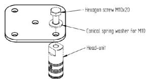
Aluminum terminal plate for external mounting of HVC conductor on air termination post
